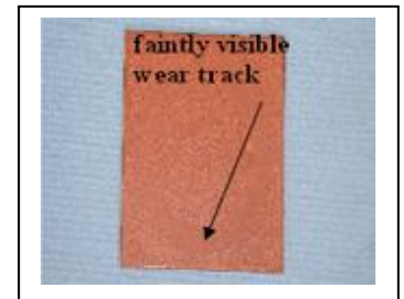
UV + room temperature cured sol-gel coated carbon epoxy substrate showing a water contact angle of 110°
